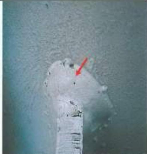
Photographic record showing Porosity at 10 o'clock Anchor Bolt Housing facing up hill on Tower 9.
