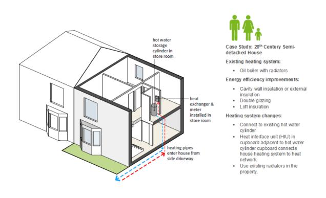
Figure 2: Example house connected to district heating Source: Ricardo Energy & Environment/John Gilberts Architect
