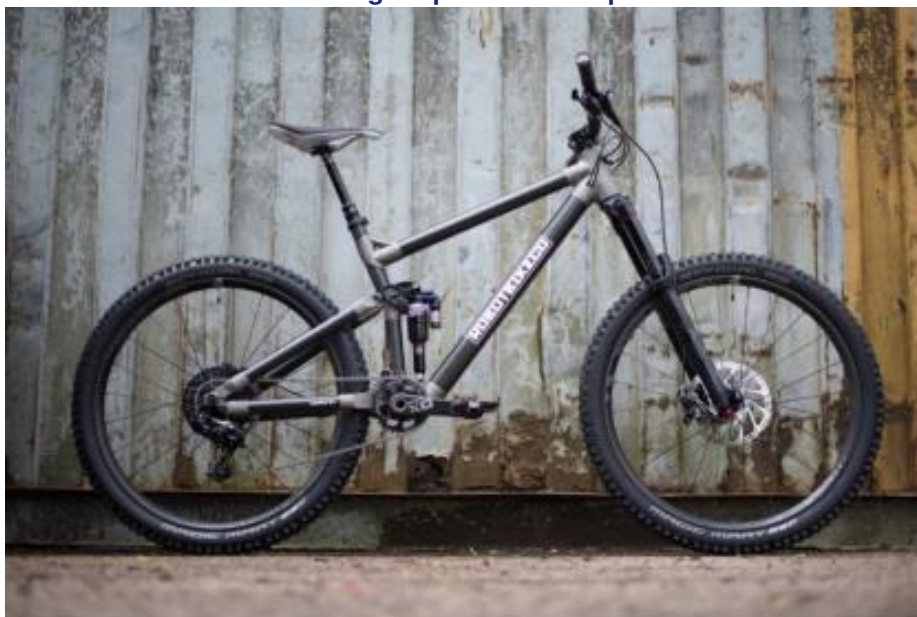
Figure 2.21 Customised bike frame using 3D printed metal parts
