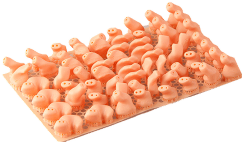
Figure 2.22 Mass customised 3D printed hearing aids
