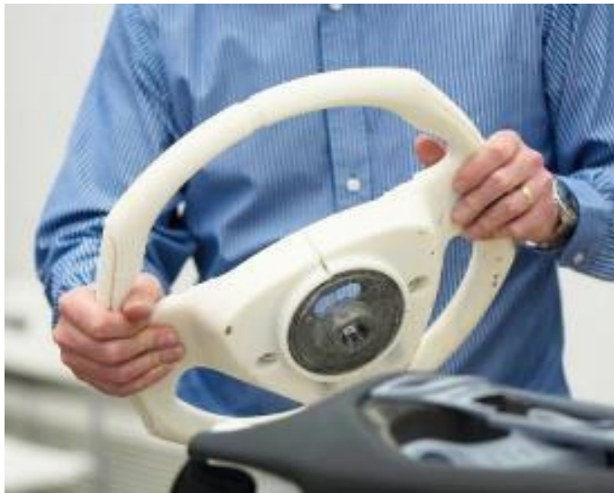
Figure 2.11 A 3D print of an Aston Martin steering wheel
