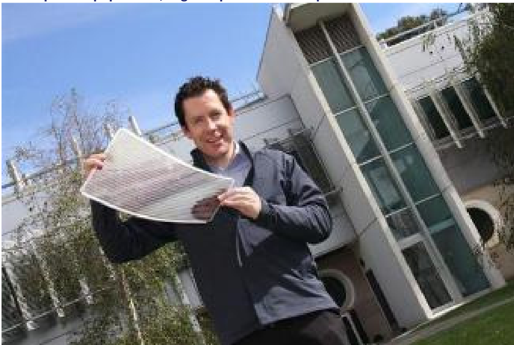
Figure 3.2 3D printed paper-thin, organic printable solar panel
