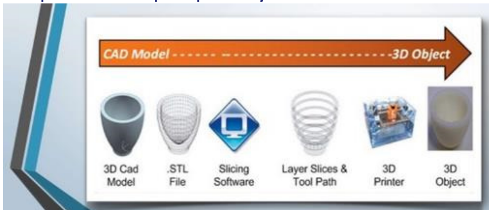
Figure 2.1 Steps taken to develop a 3D printed object
