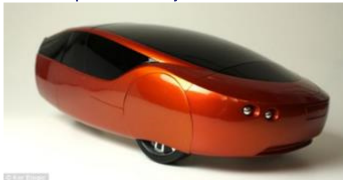
Figure 2.12 The world’s first 3D printed car body on the Urbee
