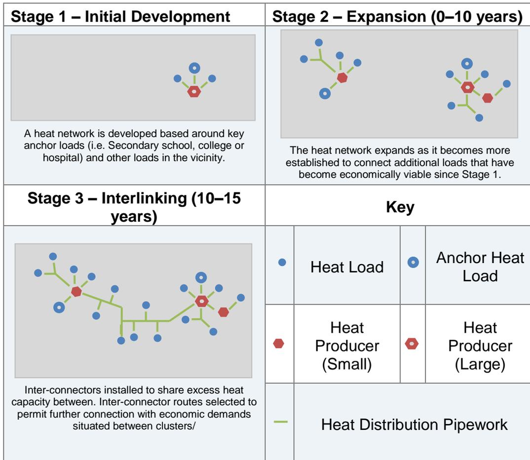
Figure 3: Stages of development of a district heating network:
