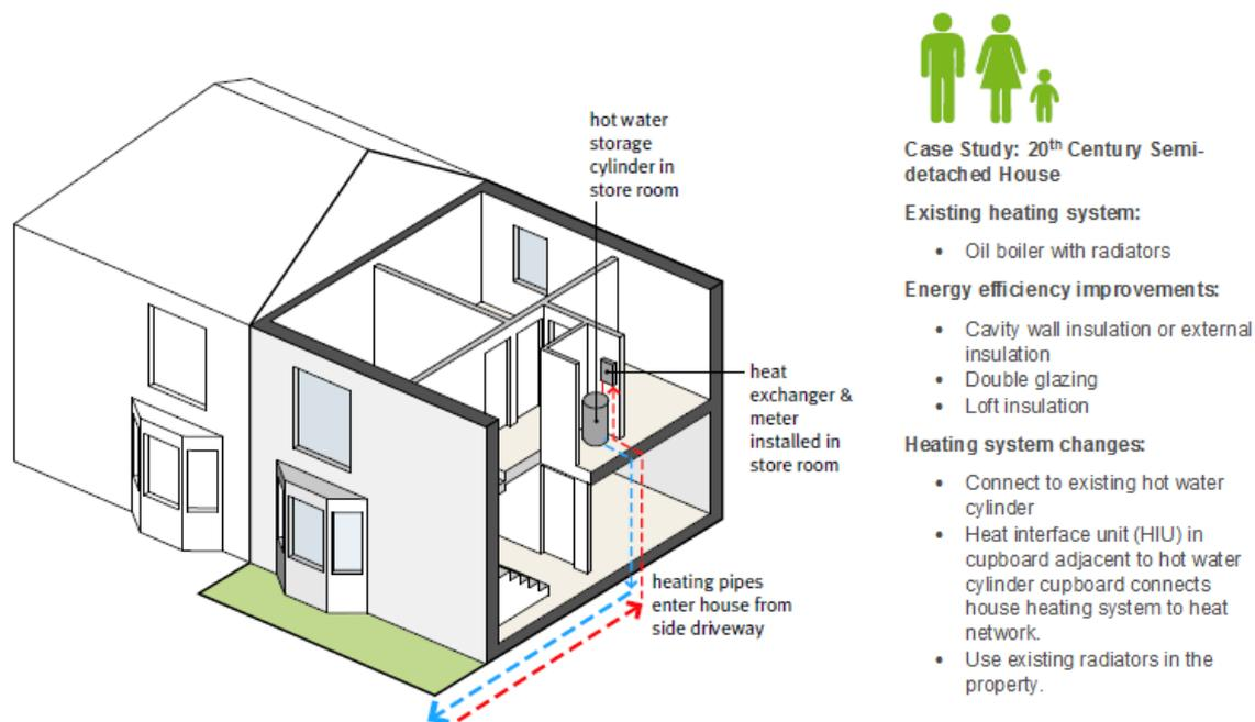
Figure 2: Example house connected to district heating Source: Ricardo Energy & Environment/John Gilberts Architect
